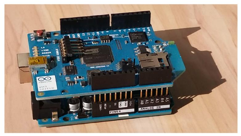
Arduino Uno with the Arduino WiFi Shield
