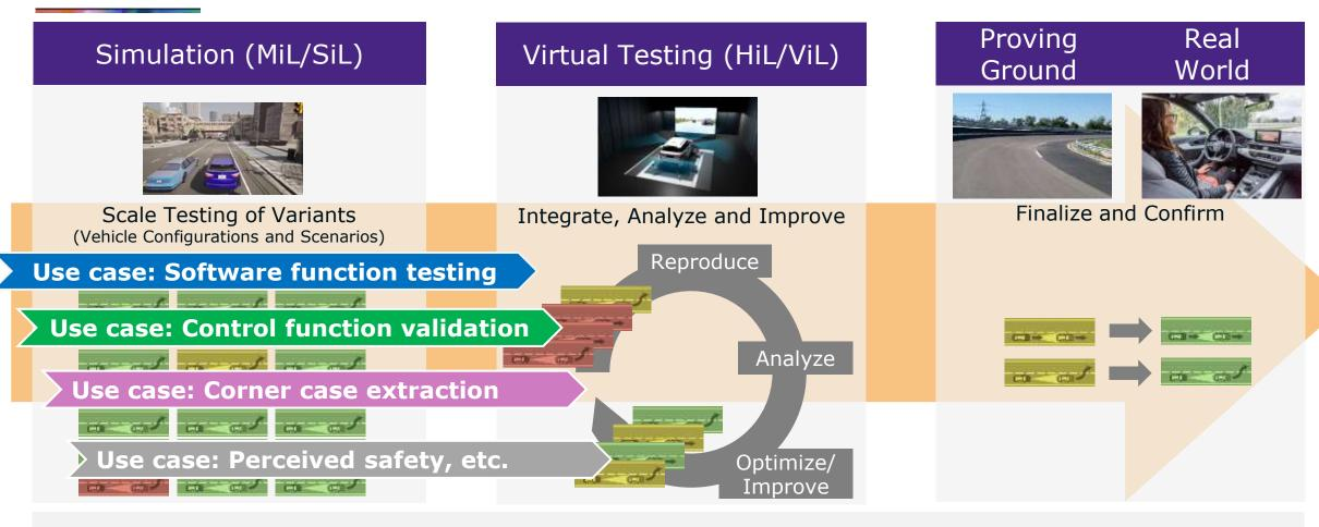
ADAS/AD function verification and validation starts in a fast and scalable virtual environment. For the higher accuracy and specific corner cases, the tests are performed in HiL and ViL environment and end up in the road tests. Validation workflow must be optimized for specific use cases in order to improve test coverage and reduce road testing.
